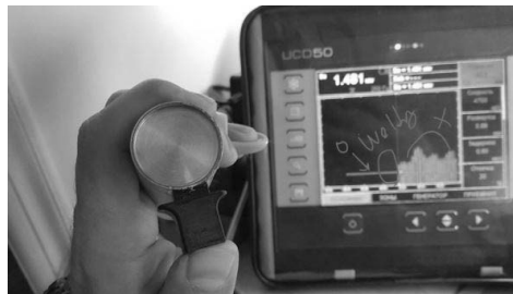
Fig. 3 – Signal spectra obtained during the study of a welded joint on a cylindrical product
