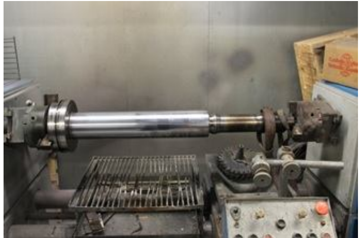
Fig. 4. A detail requiring renovation in a rotary drive
