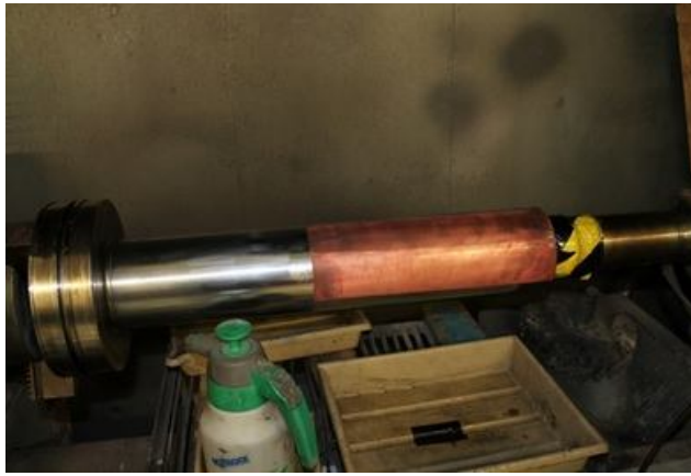
Fig. 5. Copper-based surface finish for concreting
