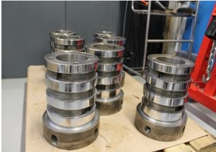
Fig. 7. Correction of local defects in stepped details
