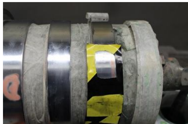
Fig. 3. Local renovation of surface defects of large-sized parts gas dynamic spray
